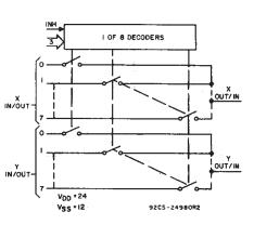
Fig. 2-CD4097 functional diagram.
