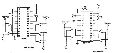
Fig. 8—Input voltage—measure  $\leq$  2  $\mu$ A on all OFF channels (e.g., channel 12).
