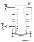
Fig. 7-OFF channel leakage current-any channel OFF.
