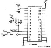
Fig. 11—Turn-on and turn-off propagation delay—address select input to signal output (e.g. measured on channel 0).
