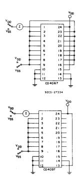
Fig. 9-OFF channel leakage current-all channels OFF.
