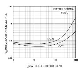
Figure 4. Collector-Emitter Saturation Voltage
