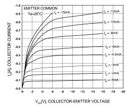
Figure 1. Static Characteristic
