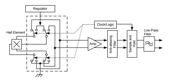
Concept of Chopper Stabilization Technique
