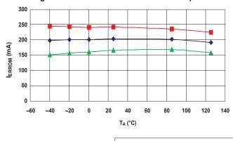
**Total Output Error versus Ambient Temperature**
