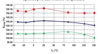
**Magnetic Offset Error versus Ambient Temperature**
