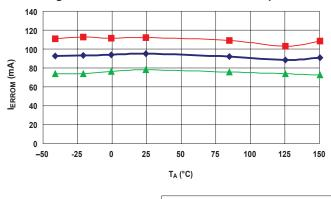
**Total Output Error versus Ambient Temperature**
