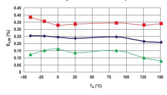
**Symmetry versus Ambient Temperature**
