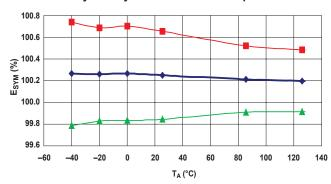
**Magnetic Offset Error versus Ambient Temperature**
