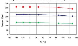
**Total Output Error versus Ambient Temperature**
