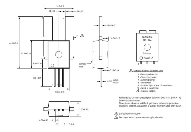
Creepage distance, current terminals to signal pins: 7.25 mm Clearance distance, current terminals to signal pins: 7.25 mm Package mass: 4.63~g typical
