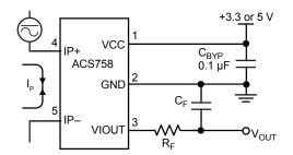
Application 1. The ACS758 outputs an analog signal,  $V_{OUT}$ , that varies linearly with the uni- or bi-directional AC or DC primary sampled current,  $I_P$ , within the range specified.  $C_F$  is for optimal noise management, with values that depend on the application.
