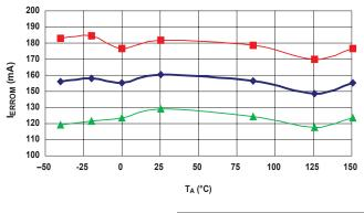
**Total Output Error versus Ambient Temperature**
