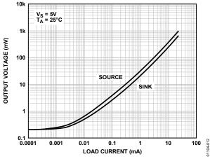
Figure 12. Output Voltage to Supply Rail vs. Output Current at 5  $\rm V$
