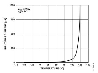
Figure 14. Input Bias Current vs. Temperature
