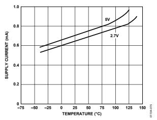
Figure 15. Supply Current vs. Temperature
