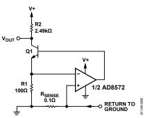
Figure 68. Low-Side Load Current Monitor
