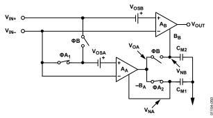
Figure 50. Auto-Zero Phase of the Amplifier
