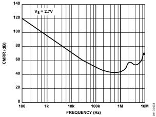
Figure 32. CMRR vs. Frequency at 2.7 V
