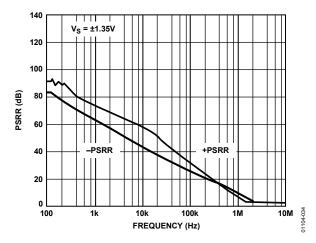
Figure 34. PSRR vs. Frequency at  $\pm 1.35 \, V$
