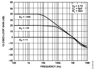
Figure 19. Closed-Loop Gain vs. Frequency at 2.7 V
