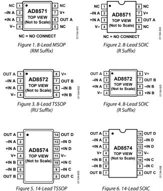
5. 14-Lead TSSOP Figure 6. 14-Lead SOIC (RU Suffix) (R Suffix)
