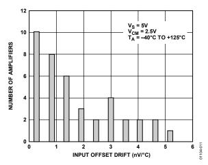
Figure 11. Input Offset Voltage Drift Distribution at 5 V
