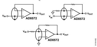
Figure 52. Guard Ring Layout and Connections to Reduce PCB Leakage Currents
