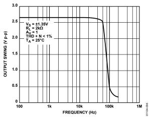
Figure 36. Maximum Output Swing vs. Frequency at 2.7  $\rm V$
