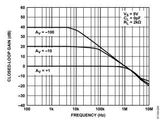
Figure 20. Closed-Loop Gain vs. Frequency at 5 V
