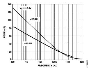
Figure 35. PSRR vs. Frequency at ±2.5 V
