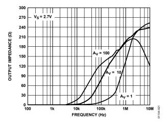
Figure 21. Output Impedance vs. Frequency at 2.7 V
