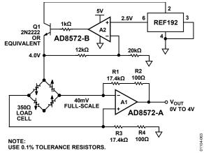
Figure 63. 5 V Precision Strain Gage Amplifier
