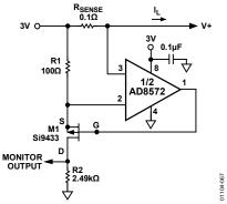
Figure 67. High-Side Load Current Monitor
