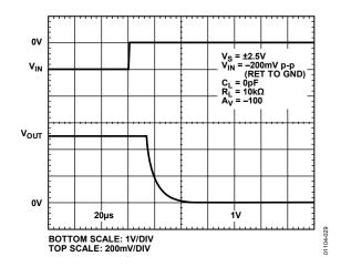
Figure 29. Positive Overvoltage Recovery
