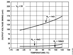
Figure 49. Output Voltage to Supply Rail vs. Temperature
