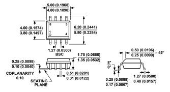
COMPLIANT TO JEDEC STANDARDS MS-012-A A CONTROLLING DIMENSIONS ARE IN MILLIMETERS; INCH DIMENSIONS (IN PARENTHESES) ARE ROUNDED-OFF MILLIMETER EQUIVALENTS FOR REFERENCE ONLY AND ARE NOT APPROPRIATE FOR USE IN DESIGN.
