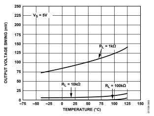
Figure 48. Output Voltage to Supply Rail vs. Temperature
