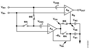
Figure 51. Output Phase of the Amplifier
