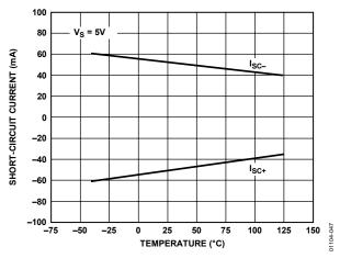
Figure 47. Output Short-Circuit Current vs. Temperature
