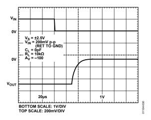
Figure 30. Negative Overvoltage Recovery
