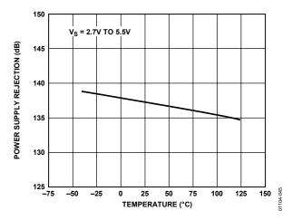
Figure 45. Power Supply Rejection vs. Temperature
