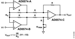
Figure 65. Discrete Instrumentation Amplifier Configuration
