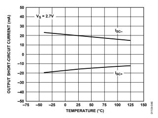
Figure 46. Output Short-Circuit Current vs. Temperature
