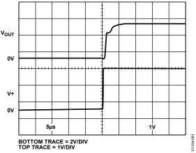
Figure 61. AD857x Output Behavior on Power-Up
