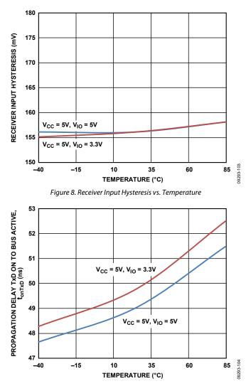
Figure 9. Propagation Delay from TxD On to Bus Active vs. Temperature
