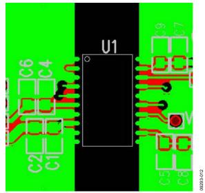
Figure 28. Recommended PCB Layout
