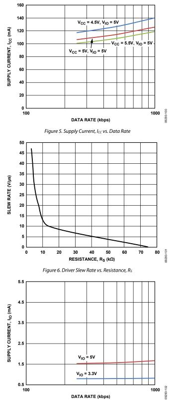
Figure 7. Supply Current,  $I_{IO}$  vs. Data Rate
