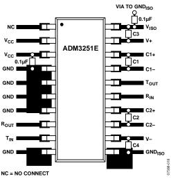
Figure 21. Recommended Printed Circuit Board Layout
