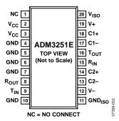
Figure 2. Pin Configuration
