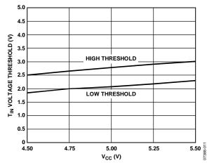
Figure 12.  $T_{IN}$  Voltage Threshold vs.  $V_{CC}$
