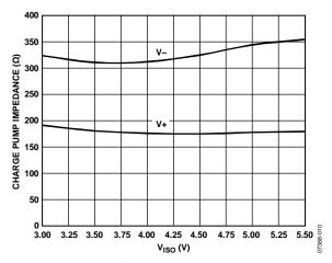
Figure 9. Charge Pump Impedance vs. V<sub>ISO</sub>
