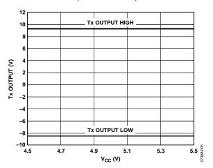
Figure 4. Transmitter Output Voltage High/Low vs.  $V_{CG}$ ,  $R_L = 3 \text{ k}\Omega$
