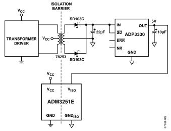
Figure 22. Isolated Power Supply Circuit
