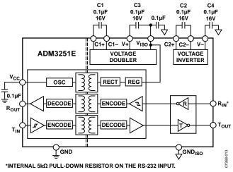
Figure 13. Functional Block Diagram
