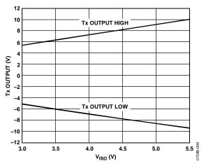
Figure 5. Transmitter Output Voltage High/Low vs.  $V_{ISO}$ ,  $R_L = 3 \text{ k}\Omega$
