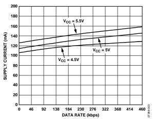
Figure 10. Primary Supply Current vs. Data Rate
