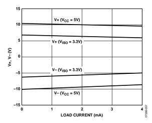
Figure 7. Charge Pump V+, V- vs. Load Current
