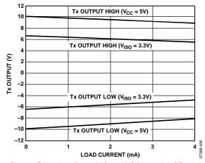
Figure 6. Transmitter Output Voltage High/Low vs. Load Current
