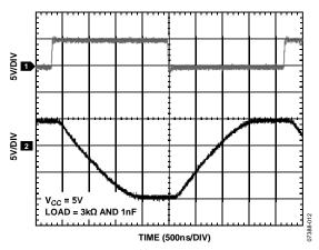
Figure 11. 460 kbps Data Transmission
