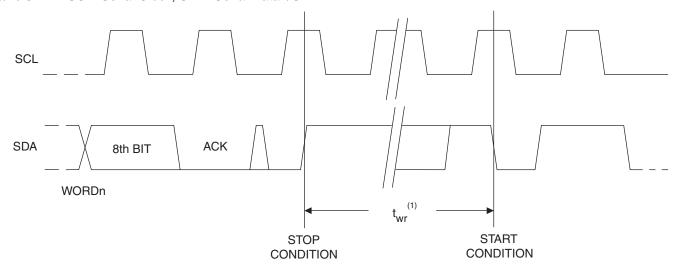
Note: 1. The write cycle time  $t_{WR}$  is the time from a valid stop condition of a write sequence to the end of the internal clear/write cycle.
