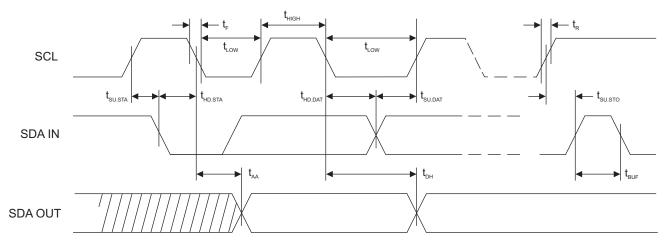
Figure 6-3. Write Cycle Timing
