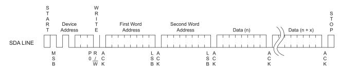
**Acknowledge Polling:** Once the internally timed write cycle has started and the EEPROM inputs are disabled, Acknowledge Polling can be initiated. This involves sending a Start condition followed by the device address word. The read/write bit is representative of the operation desired. Only if the internal write cycle has completed will the EEPROM respond with a zero, allowing a new read or write sequence to be initiated.
