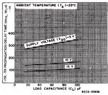
Fig. 6 - Typical propagation delay time as a function of load capacitance (+TR or -TR to Q or  $\overline{Q}$ ).
