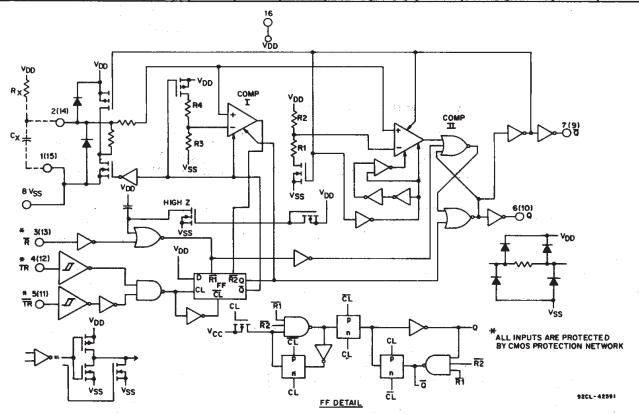
Fig. 1 - Logic diagram (½ of device shown).
