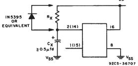
Fig. 17 - Rapid power-down protection circuit.
