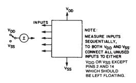
Fig. 15 - Input leakage-current test circuit.
