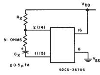
Fig. 18 - Alternate rapid power-down protection circuit.
