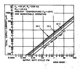
Fig. 12 - Typical total supply current as a function of output duty cycle.
