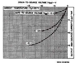
Fig. 5 - Minimum output high (source) current characteristics.
