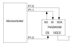
Figure 3. System Configuration without SPI port
