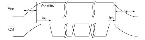
**Power Cycle Timing** ( $T_A = -40^{\circ} \text{ C}$  to  $+85^{\circ} \text{ C}$ ,  $V_{DD} = 2.7 \text{ V}$  to 5.5 V unless otherwise specified)
