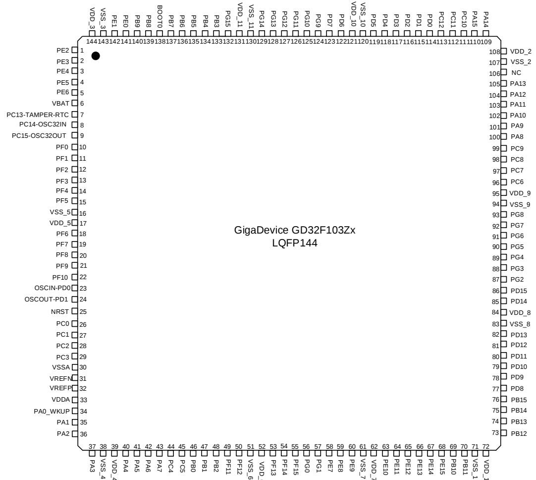
Figure 2-3. GD32F103Zx LQFP144 pinouts
