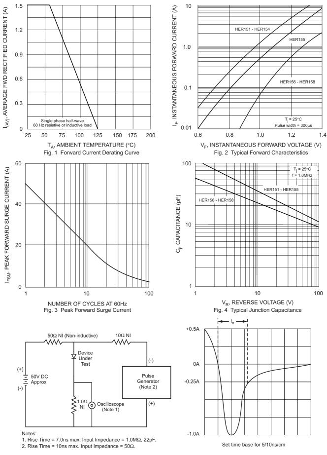
Fig. 5 Reverse Recovery Time Characteristic and Test Circuit
