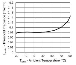
Fig. 9 - Sensitivity vs. Ambient Temperature
