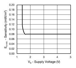
Fig. 12 - Sensitivity vs. Supply Voltage
