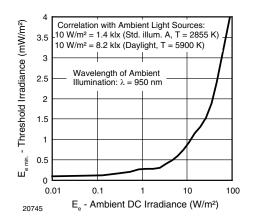
Fig. 6 - Sensitivity in Bright Ambient
