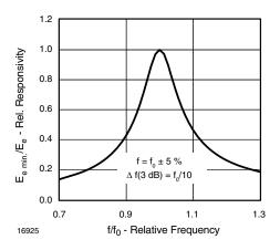
Fig. 5 - Frequency Dependence of Responsivity
