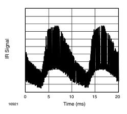
Fig. 14 - IR Signal from Fluorescent Lamp with High Modulation
