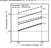
4-(2) Influence of adjacent mounting Tested sample: DS2Y-S-DC12V, 10 pcs. Ambient temperature: 20°C 68  $^\circ$  F
