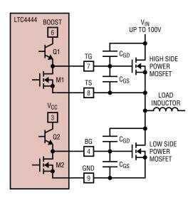
Figure 1. Capacitance Seen by BG and TG During Switching
