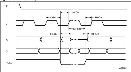
Figure 24. Output timing
