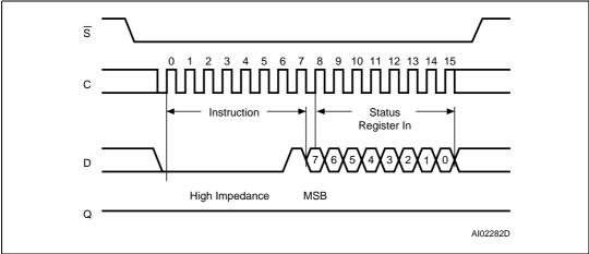
Figure 12. Write Status Register (WRSR) instruction sequence
