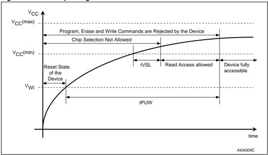
Table 8. Power-Up timing and VWI threshold
