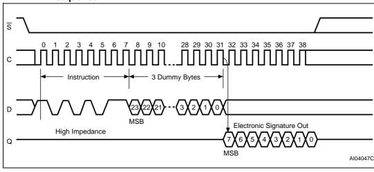
Figure 18. Read Electronic Signature (RES) instruction sequence and data-out sequence
