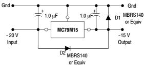
Figure 2. Protection Diodes
