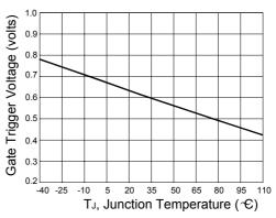
Figure 2. Typical Gate Trigger Voltage Versus Junction Temperature
