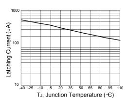
Figure 4. Typical Latching Curent Versus
