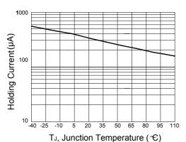
Figure 3. Typical Holding Curent Versus
