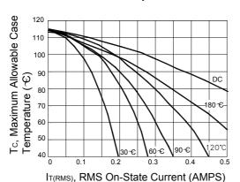
Figure 5. Typical RMS Current Derating
