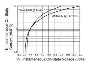
Figure 6. Typical On-State Characteristics
