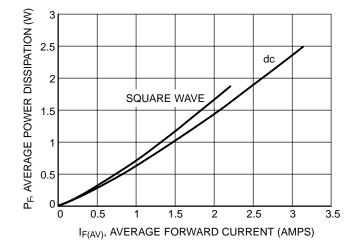
Figure 9. Power Dissipation
