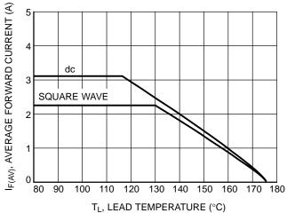
Figure 7. Current Derating, Lead
