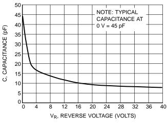
Figure 5. Typical Capacitance
