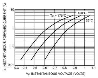
Figure 4. Maximum Forward Voltage
