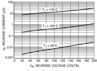
**Figure 1. Typical Reverse Current**
