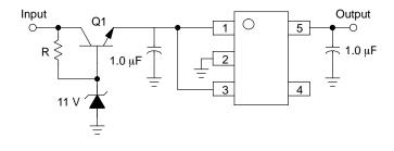
Figure 24. Input Voltages Greater than 12 V
