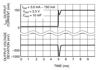
Figure 14. Load Transient Response OFF
