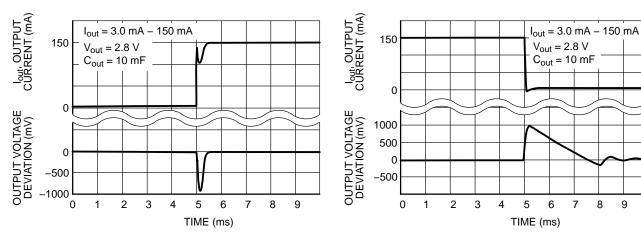
Figure 12. Load Transient Response ON
