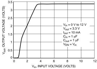
Figure 18. Output Voltage versus Input Voltage
