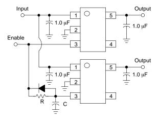
Figure 23. Delayed Turn-on
