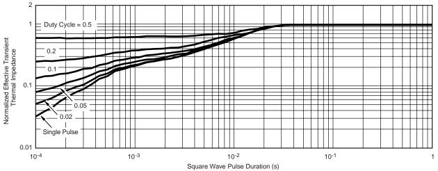
Normalized Thermal Transient Impedance, Junction-to-Case
