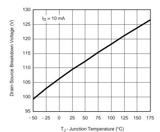
Drain-Source Breakdown Voltage vs. Junction Temperature
