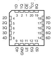
A buffered output-enable  $(\overline{OE})$  input can be used to place the eight outputs in either a normal logic state (high or low logic levels) or the high-impedance state. In the high-impedance state, the outputs neither load nor drive the bus lines significantly. The high-impedance state and increased drive provide the capability to drive bus lines without need for interface or pullup components.
