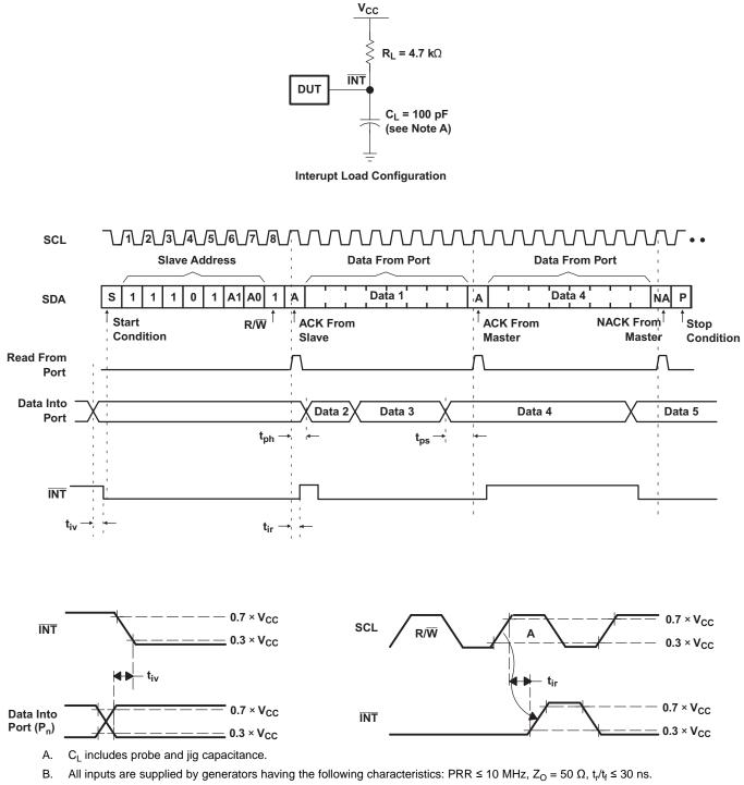
C. All parameters and waveforms are not applicable to all devices.
