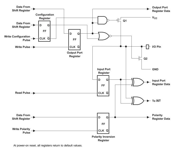
Figure 23. Simplified Schematic of P-Port I/Os
