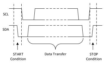
Figure 24. Definition of Start and Stop Conditions
