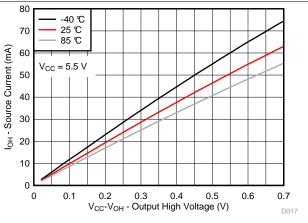
Figure 16. I/O Source Current vs Output High Voltage for Different Temperature ( $T_A$ ) for V<sub>CC</sub> = 5.5 V
