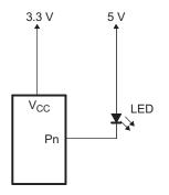
Figure 36. Device Supplied by Lower Voltage
