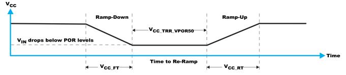
Figure 40.  $V_{cc}$  is Lowered Below the POR Threshold, then Ramped Back Up to  $V_{cc}$
