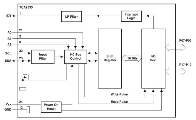
Pin numbers shown are for the PW package. All I/Os are set to inputs at reset.
