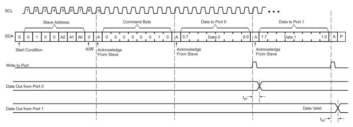
Figure 28. Write to Output Port Registers
