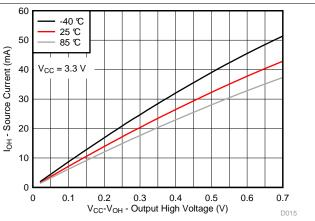
Figure 14. I/O Source Current vs Output High Voltage for Different Temperature ( $T_A$ ) for V<sub>CC</sub> = 3.3 V
