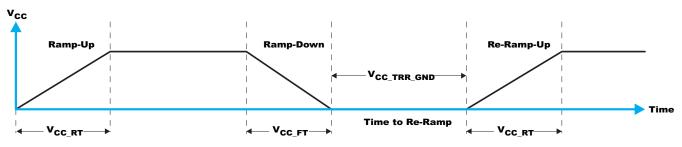
Figure 39.  $V_{CC}$  is Lowered Below 0.2 V or 0 V and then Ramped Up to  $V_{CC}$
