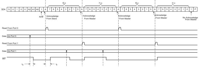
Transfer of data can be stopped at any time by a Stop condition. When this occurs, data present at the latest acknowledge phase is valid (output mode). It is assumed that the command byte previously has been set to 00 (read Input Port register).
