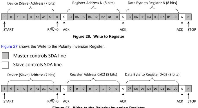
Figure 27. Write to the Polarity Inversion Register
