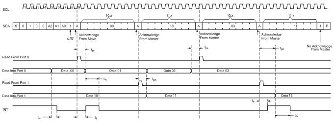
Transfer of data can be stopped at any time by a Stop condition. When this occurs, data present at the latest acknowledge phase is valid (output mode). It is assumed that the command byte previously has been set to 00 (read Input Port register).
