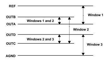
Figure 13. Overlapping Window Structure
