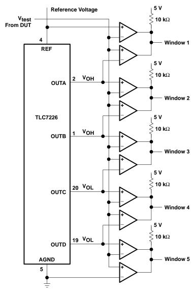
Figure 10. Logic Level Measurement
