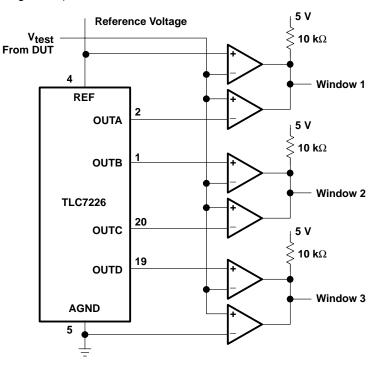
Figure 12. Overlapping Window Circuit
