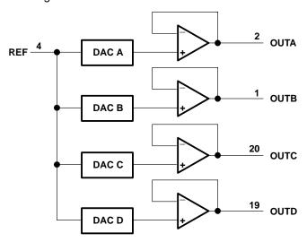
Figure 7. Unipolar Output Circuit
