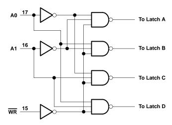
**Figure 6. Input Control Logic**
