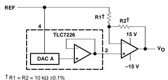
Figure 9. Bipolar Output Circuit
