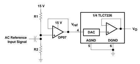
Figure 14. AC Signal Input Scheme
