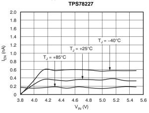
**ENABLE PIN CURRENT vs INPUT VOLTAGE**
