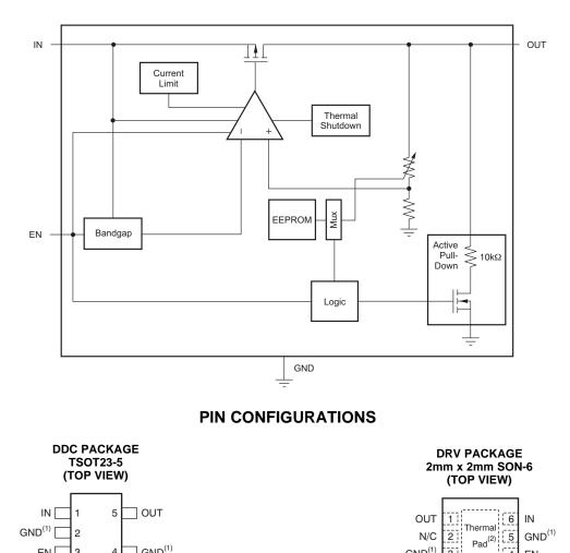
(1) All ground pins must be connected to ground for proper operation.
