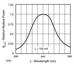
Fig. 8 - Relative Radiant Power vs. Wavelength
