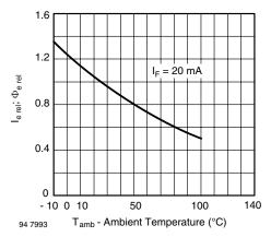
Fig. 7 - Relative Radiant Intensity/Power vs. Ambient Temperature
