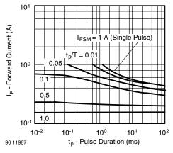
Fig. 3 - Pulse Forward Current vs. Pulse Duration
