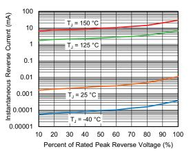
Fig. 4 - Typical Reverse Characteristics
