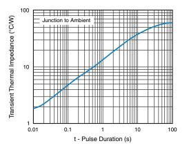
Fig. 6 - Typical Transient Thermal Impedance
