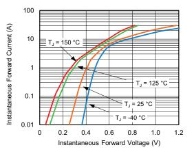
Fig. 3 - Typical Instantaneous Forward Characteristics
