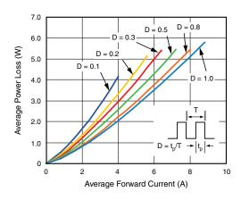
Fig. 2 - Forward Power Loss Characteristics
