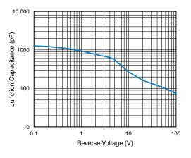
Fig. 5 - Typical Junction Capacitance
